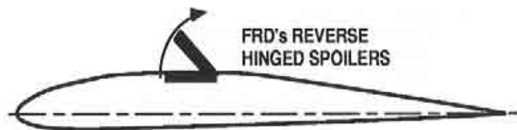
Figure 5 - Deis' Reverse Hinged Spoilers
