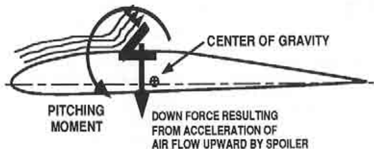
Figure 4 - Flap Type Spoilers May Produce an Additional Pitch Down Pitching Moment When Deployed
