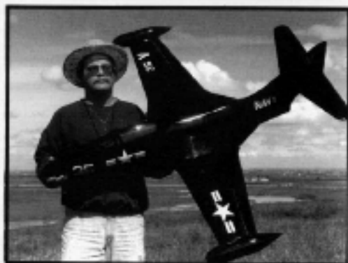
Joe Newland's F9F Panther Jet from Hangar Hobbies. Wing is 53", length 55", 6 lbs., glass fuselage, foam balsa wing.
