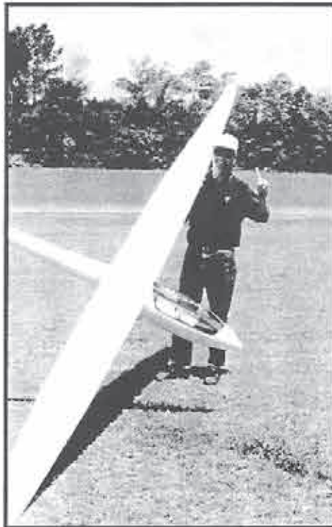
Mike Watson's 1/3 ASW 19 has unique polyhedral wing tips. It's a great thermal sailplane.
