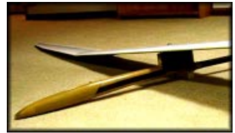
The characteristic pylon and boom construction.
