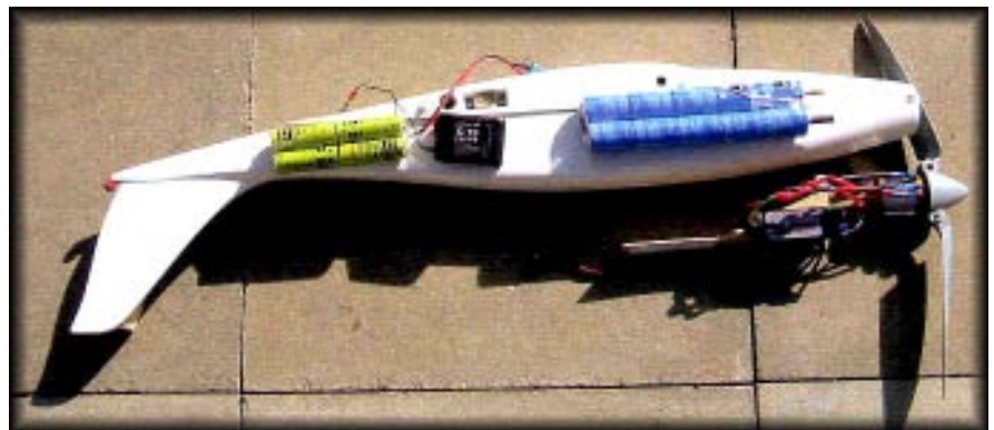
Layout of the components of the Taborca electric version.
