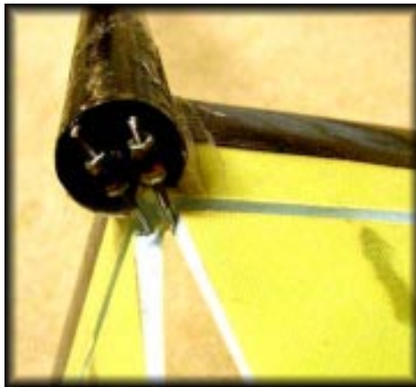
The tail from the bottom. The "horns" are made from pushrods and the pushrods are attached using ball joints. The pushrods themselves are carbon fiber running in Teflon sheaths. A major area of innovation is control horns and their attachment to the tails.
