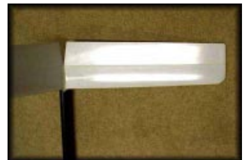
The tail from the top. Notice that the hinge line is at the 50% mark.
