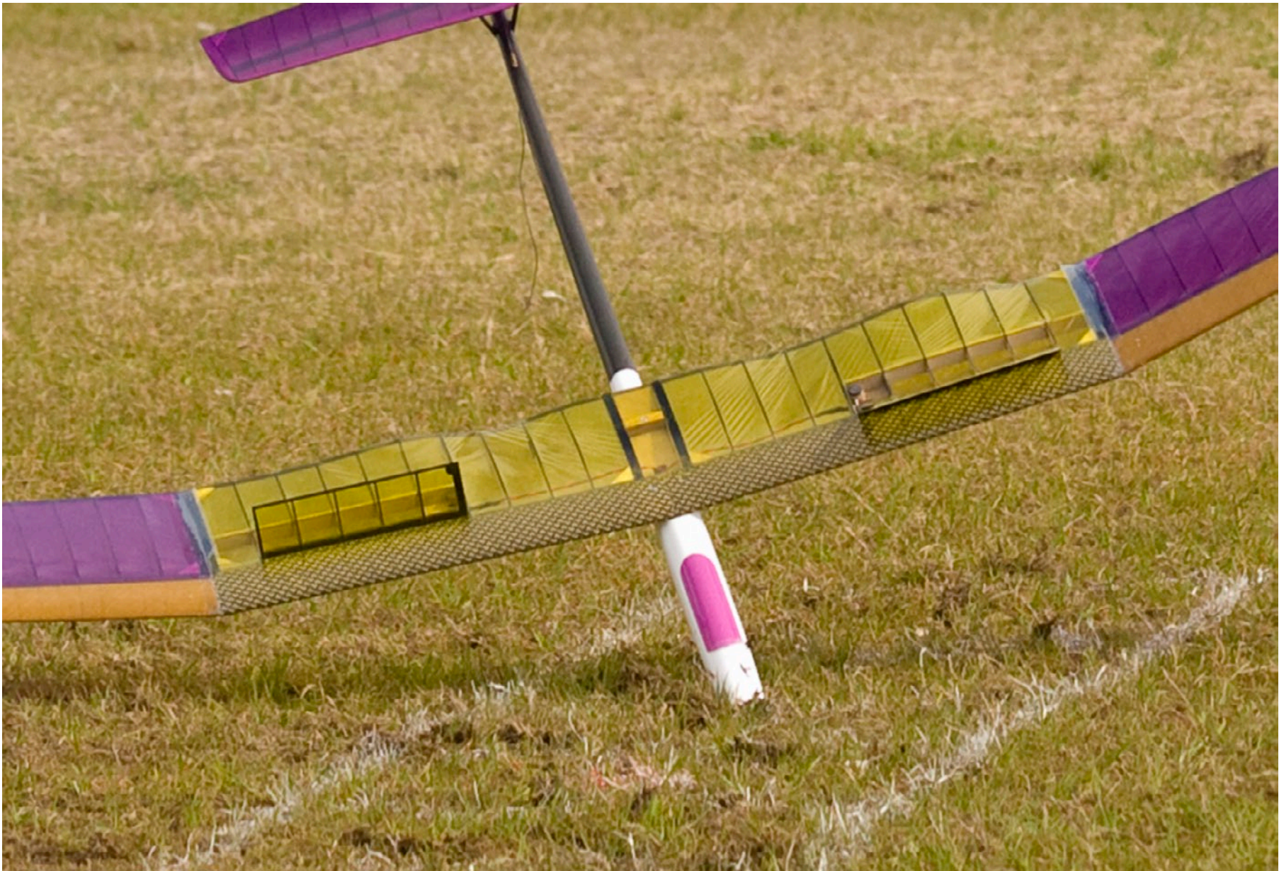
Flexible Topaz - John Erickson (Valencia, CA) “pilots” his Topaz to a landing at the 2008 South West Classic in Queen Creek, Arizona. No damage, but the extreme flexibility observed a few milliseconds after touchdown is quite astounding.
