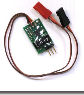
set is often not used on a sailplane. The device is switched off for most of the flight - we do not want the rudder wagging on tow, or when climbing out under electric motor power. After the sailplane enters cruise mode, and when switched on from the transmitter, it indicates rising air by gently wagging the rudder side-to-side, sensing a decrease in atmospheric pressure to detect lift.
