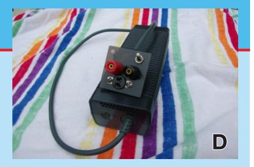
Then solder the red and blue together, or as I did add a small single pole single throw on/off switch, this tricks the PS into turning on. You know it's working because the pilot light turns from yellow to green. Now all you have to do is solder on a plug of choice and you're done, again I added the banana plugs in my case it was just that simple.
