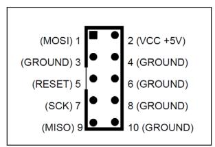
Pin out of the female IDC header on the programmer. Comparison of this image with the image showing the wiring should help reduce any confusion if following the ER9X installation instructions.
