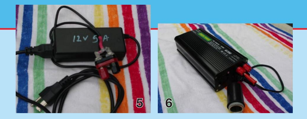
others, as the 120 VAC wiring is exposed and a cover (the red thingy) of some sorts should be added to avoid risk of electrocution.
