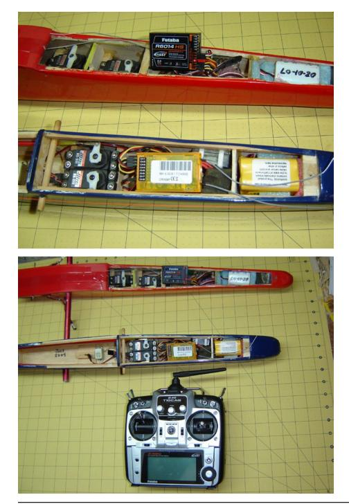
The top fuselage is a 9-servo sailplane so the 14 channel R-6014 receiver gets a workout. The Orange 2.4 GHz FASST receiver in the Oly II fuselage is about the same size as the Futaba receiver but slightly thinner. The two coaxial leads used on each receiver are identical. Current drain was also about the same for each receiver with the servos unplugged.
