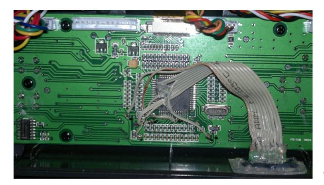
Close-up of the main board. The IDC female header detailed on the previous page is located at the lower right.
