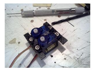
Servos mounted on carbon fiber rails.
