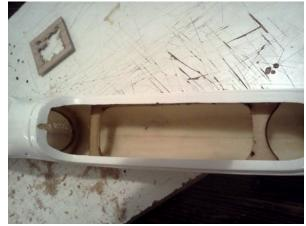
After grinding with a Dremel. Still enough left to strengthen the fuselage.
