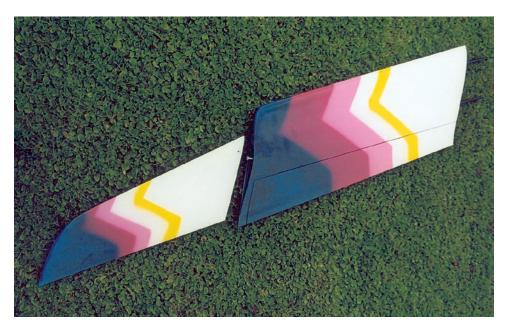
In fact, the operation of the winglets is much more complex than I have just described simplistically. In fact the not negligible increase of efficiency is also due to the fact that they change the distribution of lift increasing it at the ends.
