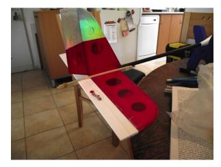
Sticks keep the elevator in neutral while setting up the pull-pull system.
