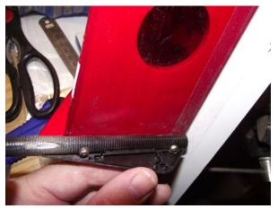
Tail group mounted to aft end of tail boom. Note the plastic skid.
