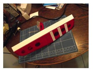
Bottom of the tail group, two mounting bolts on the stab centerline.
