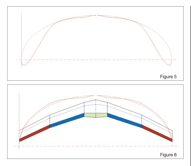
For the straight flight, the ideal was to obtain an elliptical distribution at high speed and, at the same time, avoid lift inversion in the conditions of minimum wing loading and maximum expected speed. This condition - the one to be avoided - is depicted in Figure 5, and is relative to a speed of 30 m/s with 1.5 degrees of negative tip wash-out. The condition of straight flight with 0.5 degrees of negative wash-out is instead that of Figure 6, obtained at 30 m/s.
