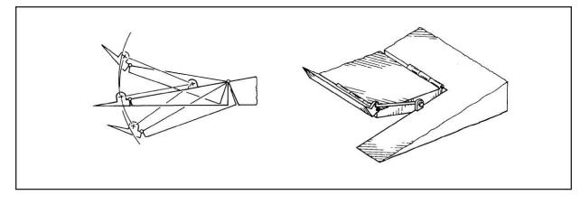
The Kasper trim device geometry forces the tab portion of the control surface upward any time the control surface is not in its neutral position Our uncertainty comes when determining how large this tab needs to be on the Windlord, so we're looking for advice from the group.
