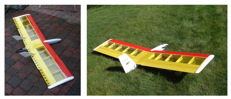
Left: The pusher configuration with twin fins, outboard ailerons and inboard elevators. Right: The tractor configuration with full span elevons. Full size plans for the Little Plank III are available at <a href="http://www.b2streamlines.com/Clemans/Little\_Plank\_III.pdf">http://www.b2streamlines.com/Clemans/Little\_Plank\_III.pdf</a>.
