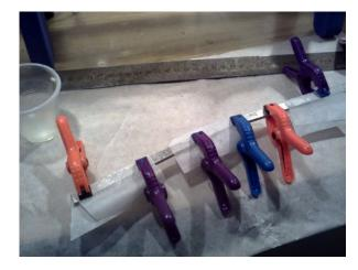
Gluing the metal spar pieces together.
