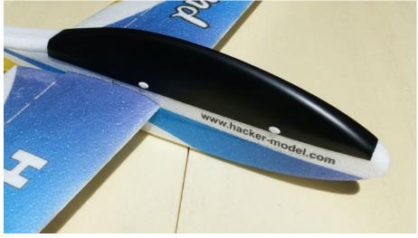
The canopy is locked with four plastics clips. These clips are glued on the canopy to not loose them.
