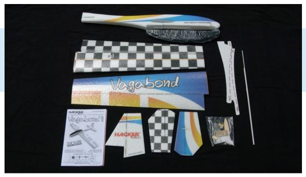
installation. The fuselage, however, needs some work, like inserting the carbon rods for stiffness, the sleeves for the rudder and elevator control rods, the servo tray, the root section in the middle of the fuselage, the fin and the tailplanes.
