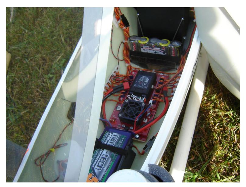
This is the radio room of Steves sailplane. The radio is JR with satellite receivers installed to assure rock solid reception. The radio and servos are powered by the enormous LiPo batteries (2) that are mounted just
