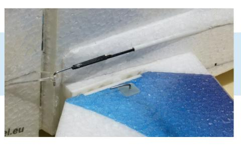
The rudder linkage end, and the lock L shape clip added to the tailplane to make it removable.
