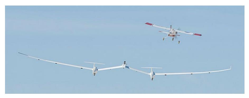
One of NASA Armstrong's DROID small unmanned research aircraft tows the twin-fuselage towed glider into the blue sky on its first test flight.
