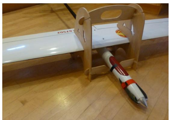
Jim Loughran used his CNC machine to cut ours out of 6mm plywood. I would think that cutting and sanding by hand using the Adobe plans (pdf) would work well, too.
