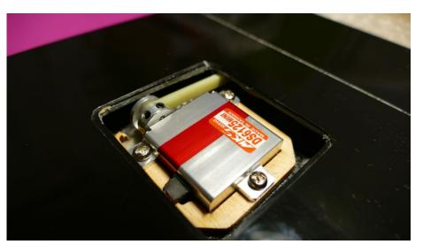
Rotmilan\_21: The servo and LDS system in place in the wing. No slop at all !
