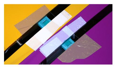
The risky step of the gluing of the green connectors in the wing root. I used PVA release agent everywhere it was needed, in addition to some thin tape to protect the fuselage and the root of the wing.
