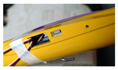
The wire routing in the fuselage is tight and requires some attention. To strength the connector fixation, I built an upper and lower side to side tray with thin plywood
