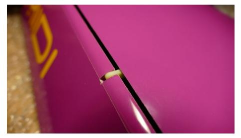
The control rod is fiberglass and totally integrated into the wing
