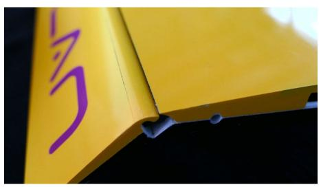
Wipers are molded at the same time than the rest of the wing, which means that ailerons/flaps are position with an angle in the molds.
