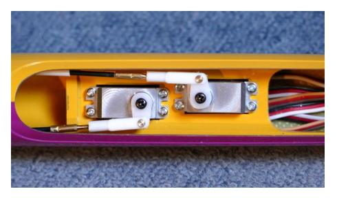
I like the MPjet plastic clevises, because they are tight on the coupler and suppress the slop at the servo arm level.
