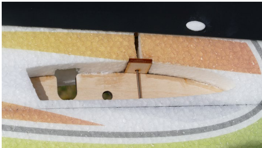
The center fuselage rib, and the small plywood part provide guidance to the lock system
