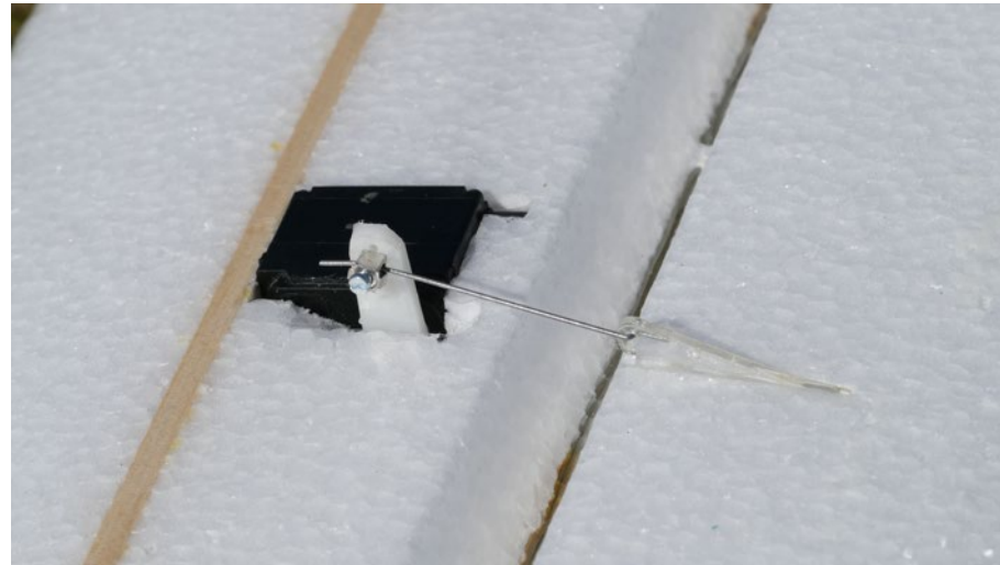
The aileron servo is a big 15 mm with plenty of torque for the large aileron
