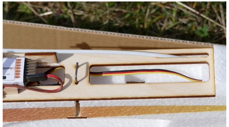
The rear part of the servo tray provides good access to catch the aileron servo wire when assembling the plane on the slope
