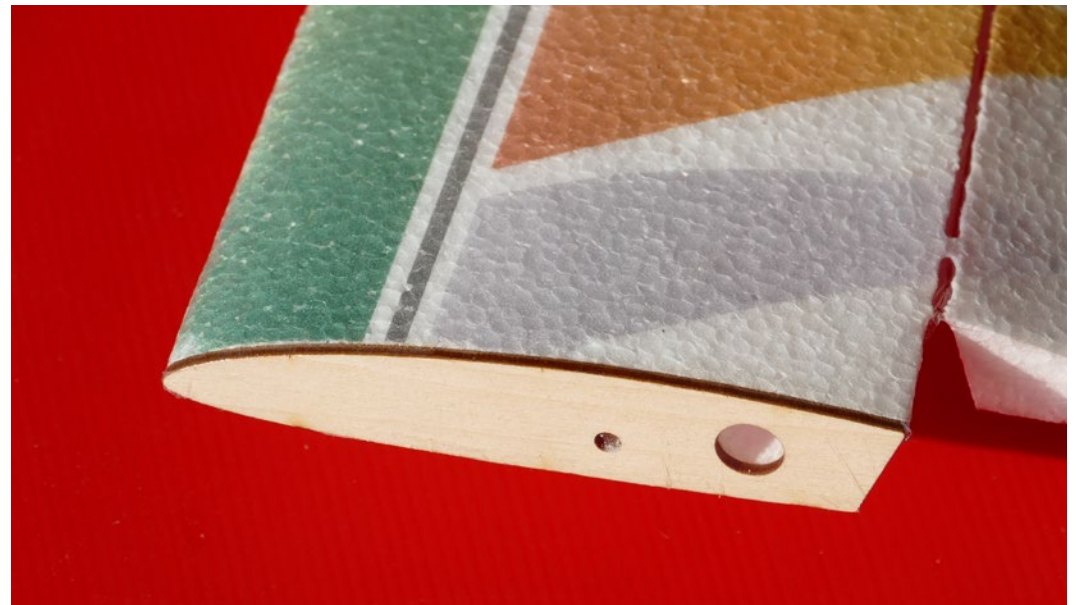
The laser cut root rib already in place on the wing
