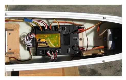
The RCCSKJ Power Box fitted with wiring almost complete.
