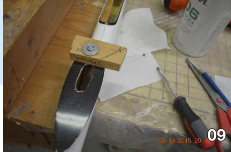
the location of the bolt and drill a hole for the T-nut just aft of the mark.
