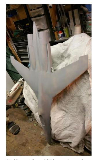
27. I braved the cold this evening and cracked on with a first guide coat of primer on the Flanker. The fins, sub fins, ailerons and elevators are now drying out with their first layer of glass too. All coming along!
