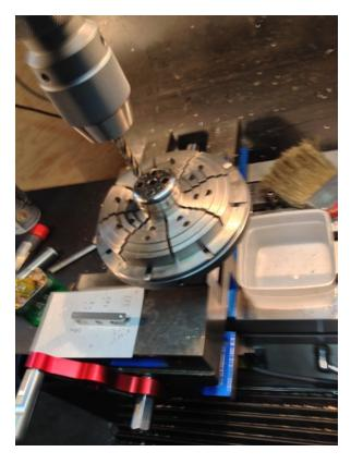
7: The cap in a fuzzy concentric chuck. The fuzziness of the photo makes a softer surface for holding the cap.
