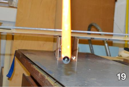
Square the fin to the wing and mark the rear wing bolt by drilling through the rear bolt pilot hole.
