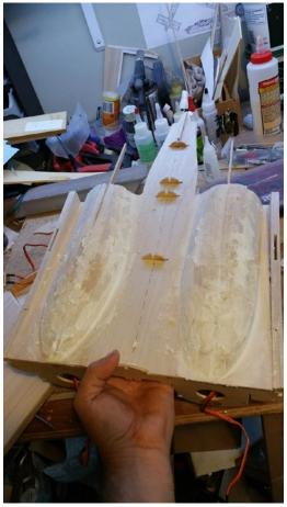
8. Some shaping has started on the engine tops now too. Heavy duty carving, then splattered with lightweight filler, as usual.
