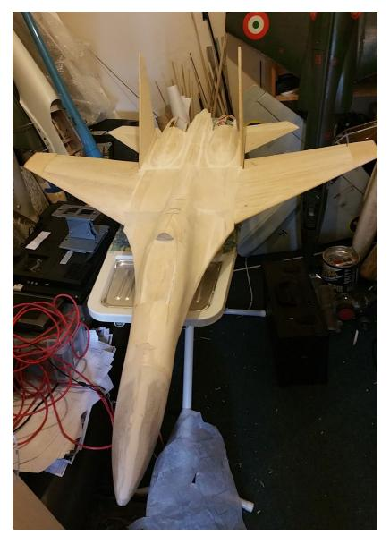
23. Here are the ailerons taped-on, with the tailset mounted too. All the wiggly bits had a final sanding last night, and hinge points added ready for when the primer is on.
