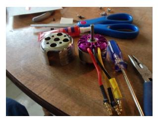
8: Milled cap & motor. I salvaged this motor from a 3D plane I shouldn't have got at an RC swap meet which came with a bad speed controller. The groove at the end of the shaft shows its shaft had been reversed.
