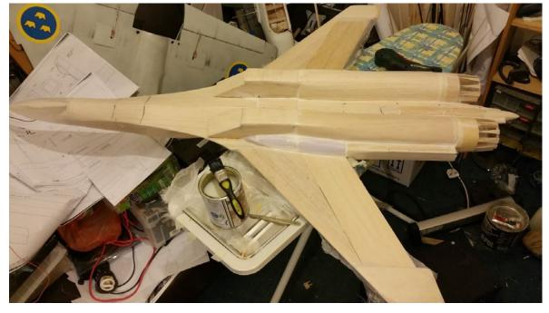
26. Well, it's hard to see here, but that's the underside of the airframe all glassed. I'm using Ronseal diamond-hard WBPC varnish, and some fairly light (no idea on weight) cloth. I really like glassing - it's so quick!
