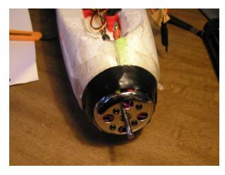
9: Martini cap and motor installed in EasyGlider Electric.
