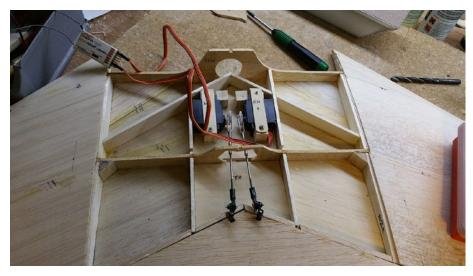
7. The Su-27 now has both tail and aileron servos installed and linkages set-up. Time to start joining these big lumps together!
