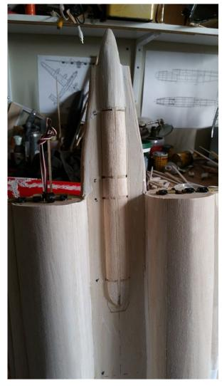
14. (Left) The build progresses nicely - lots of filler splattered here and there, a few filling blocks of pink foam squeezed in, and the sanding has started in ernest. It's all going quite well at the moment, so may even see some glass fibre applied before the year is out, which will be nice. It's all going quite well at the moment, so may even see some glass fibre applied before the year is out, which will be nice.
