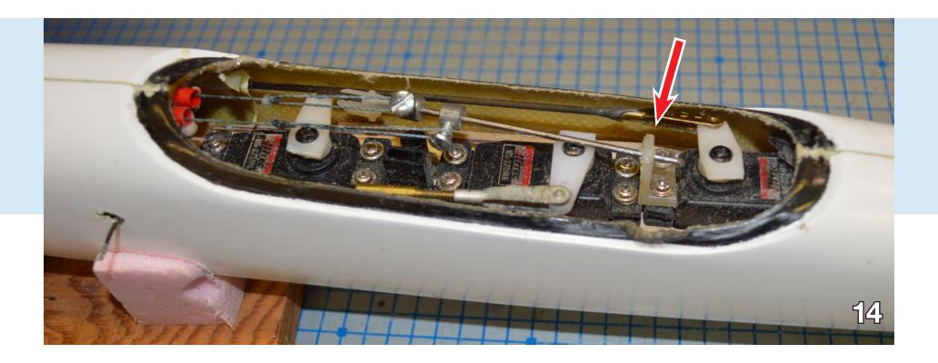
The guide tube is glued to the inside of the pylon and at the aft edge of the hatch with filled epoxy.
