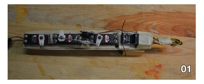
Therefore I fell back on a removable servo tray installed as far forward as possible. I mounted the XPS Nano receiver on the back of the servo tray and let servo leads extend back inside the fuselage making a removable servo and receiver package that can be worked on and tested on the work bench (Photo 01).
