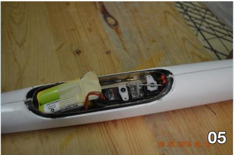
Splicing a female servo connector in the negative power lead let me use a shorting plug in the socket to connect the battery. I also use the center pin in the socket to charge the battery through an adapter made by splicing two servo leads salvaged from deceased servos to connect the charger. See the wiring diagram at right and Photo 6.
