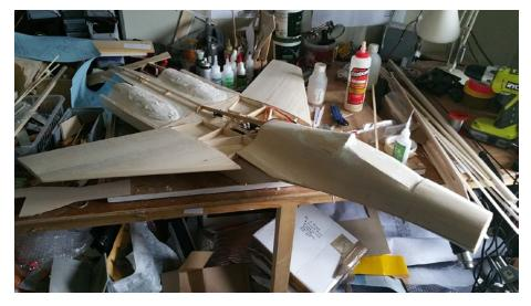
10. Here she is, now joined together. Just finishing up a few gaps in the planking and the odd balsa in-fill, then on with the major sheeting.
