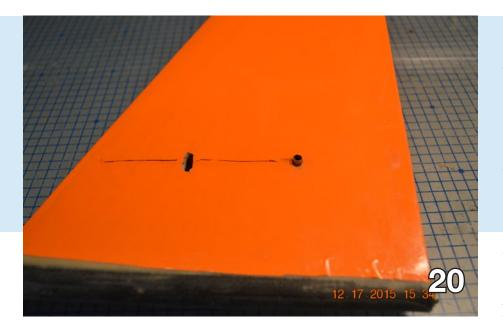
The stab pivot bearing is 5/32 inch brass tubing and should extend about 1/16 inch outside the fin to proved a gluing surface (Photo 20). Add a 1/8 inch soft balsa rib to the stab root with a 5/32 hole for the stab bearing and sand to match the fin contour.
