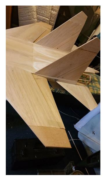
24. The wing tips have had the 1/16th inch ply end plates added to stiffen things up, and also hold the removable missile rails.
