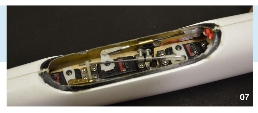
Since the receiver is not accessible for inserting the binding plug, I use a remote bind button. "Two Useful Gadgets" in the March 2015 issue of *RC Soaring Digest* shows how I did it.
