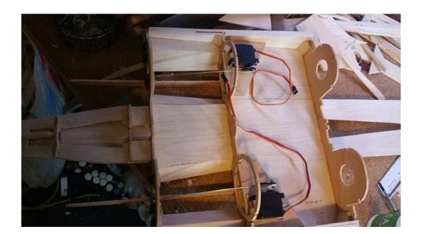
6. Here is a picture of the separate all-flying-tail servos installed in the underside of the tail section of the Su27.
