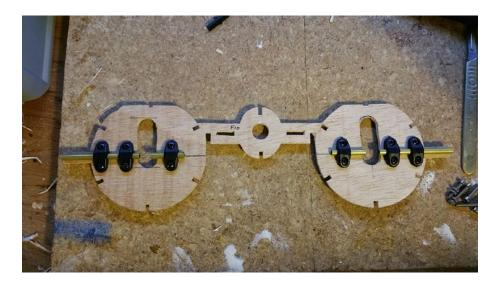
3. The construction of the rear fuselage continues, here you can see tailplane mechanism going into the rearmost liteply former.
