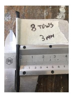
1. Start by laying out the appropriate lengths of carbon fiber tow. This 12K carbon tow is looped to form six lengths of about 1 meter.
