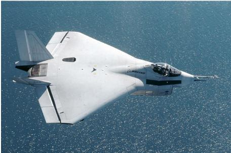
http://notreally.info/transport/planes/jsf/x-32/img/x-32\_Boeing-X-32-medium.jpg X-32B from above. No leading edge devices, shorter span.
