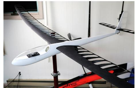
The wings and stabs repaired and ready to cover. Sprayed the wood with flat black paint to hide the plywood which was stained orange from the original Monokote. I think a black stain would have worked better as the Ultracote covering adhesive interacted with the flat paint and caused blemishes.
