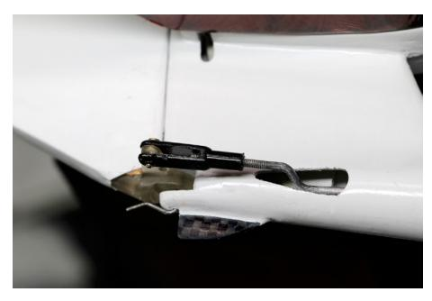
On my model the tail skid which also secures the rudder keeper pin was missing completely. I fabricated a new tang and tail skid to hold the wire in place. Replaced the ancient nylon clevis with a MP jet fork which is much stronger.
