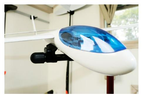
The dyed canopy really contrasts well with the white fuselage and new black carbon plate servo tray. I cover tips on the dying process in one of the videos.
