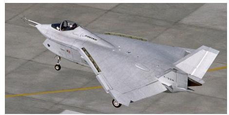
http://www.arcforums.com/forums/air/lindex.php?/topic/270399-any-chance-of-a-148-boeing-x-32/ X-32A in landing mode. Leading edge devices include leading edge flaps outboard and leading edge spoilers inboard.
