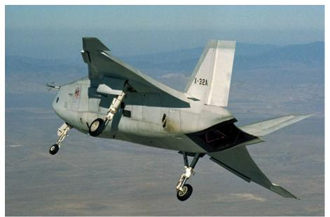
http://www.arcforums.com/forums/air/index.php?/topic/270399-any-chance-of-a-148-boeing-x-32/ The X-32A in landing mode. Note extended leading edge devices and downward deflection of elevons.
