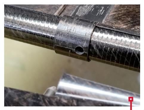
Third, there is a hole in the rear keeper. Align the hole in the boom with the hole in the rear keeper.
