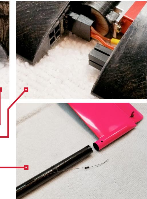
Pay attention to the detail in the online plans on where to install the pull cable keeper. The dimensions shown on the plane will make sure the keeper is installed on the wire so the keeper is past the end of the boom which makes threading boom and pull wire through the joiner and rear keepers easier to do.
