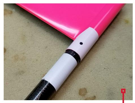
Start by covering with tape the area where you don't want the epoxy to bond to. Use a little water base jelly on the end and inside the tail where it slips over the boom.
