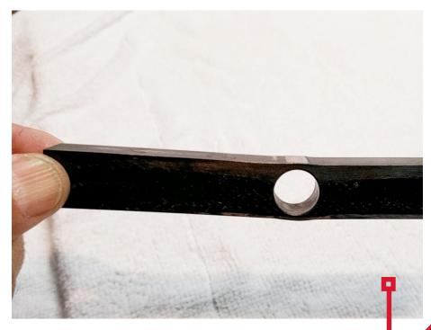
The joiner is rather unique. This allows the center wing panel, the A-tail booms and outer wing panel to all integrate into one single component, that is selfaligning and all the servos connect automatically. It is stronger than it looks.
