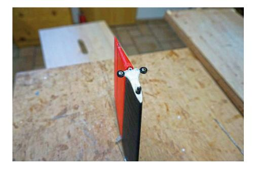
rudder is in balsa for the leading edge and ribs, linden for the side members. The servo is housed at the point of maximum thickness and moves the elevator by means of a 3x0,5 carbon tube transmission and clips. At the head of the fin there is the elevator fixing, formed by two uniball and joined with an M2 threaded rod and glued to the top of the rudder side member with a kevlar tow tie.
