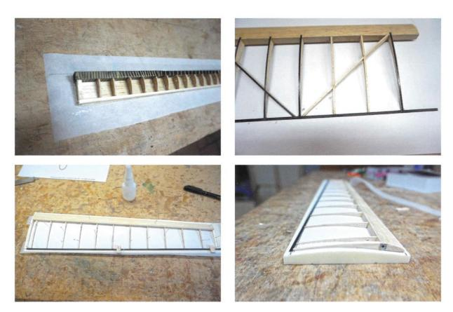
The Swift wing details: a spar and D-box close-up, first, second and third wing panels.
