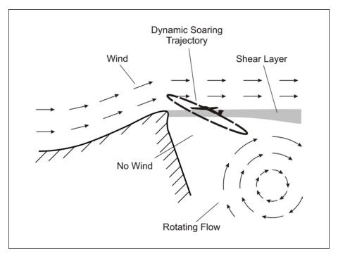
Figure 1. High-speed mode of dynamic soaring in region behind ridge.
