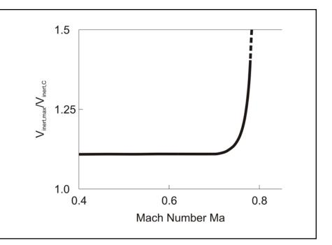
Figure 7. Effect of compressibility on the relation between  $V_{inert,max}$  and  $V_{inert,C}$  .
