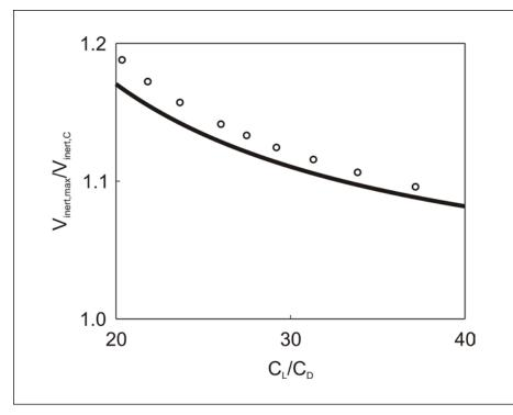
Figure 5. Dependence of speed ratio  $V_{inert,max}$  /  $V_{inert,C}$  on lift-to-drag ratio  $C_L$  /  $C_D$ .
