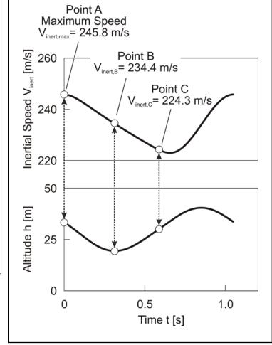
*Figure 3. Speed and altitude time histories of dynamic soaring loop optimized for maximum speed.*
