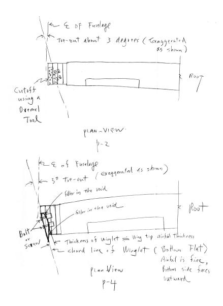
an inward lifting force is created in flight. The winglets are fiblerglassed (only at the base) and covered with heat-shrink film.
