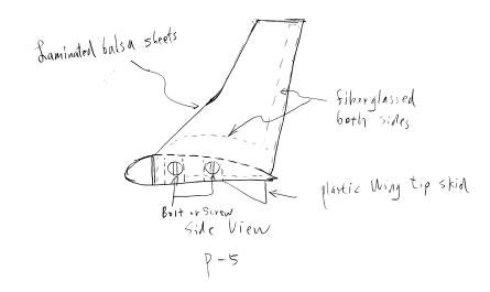
should be self-explanatory. The dimensions of the winglets: about -inch thick, about 2.5-inch at the base from LE to TE and about 3.5-inch from base to tip. The additional weight of winglets is nil for 4- meter size gliders.
