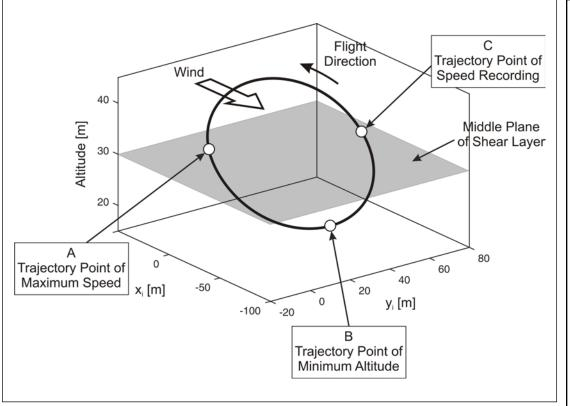
Figure 2. Dynamic soaring loop optimized for maximum speed.
