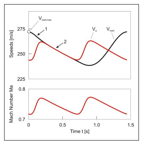
Figure 6. Time histories of  $V_{inert,max}$ ,  $V_a$  and  $M_a$  and during high-speed dynamic loop optimized for maximum speed.
