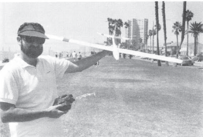
Dave Greenwood's vacuum-formed fuselage. Originally, he and Bill Salek of the La Sierra Slope Soarers designed a replacement fuse for the Talon. Now they're working on a partial kit of their own. Vacuum-formed fuse, Selig 3021 or SD6060 foam cores, it'll cost around $35.
