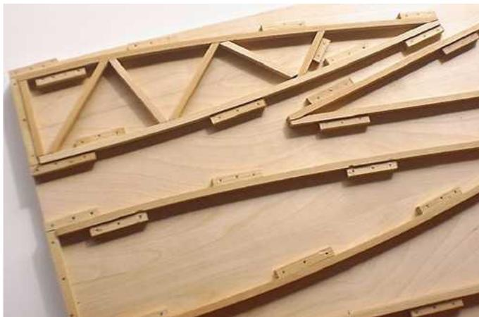
**ABOVE: Now you can see the cross pieces in place inside of the rib's outer pieces. The last step in the process is to add the gussets at each joint on both sides of the rib to provide the necessary strength and rigidity.**
