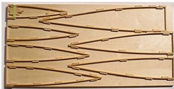
**ABOVE: This is the finished rib board with a the beginnings of a rib inserted in the restraining blocks.**
