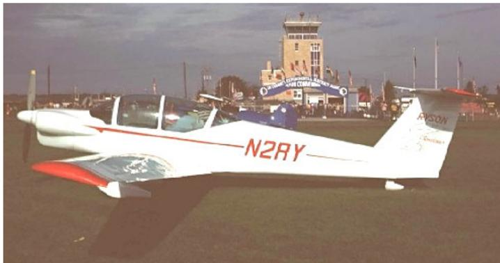
These are a couple of shots I found on the Internet of the Cloudster, but I can't tell the name of the airport. This gives you a good idea of the aircraft in the fully configured condition, including the wheel pants on both the mains and tailwheel.
