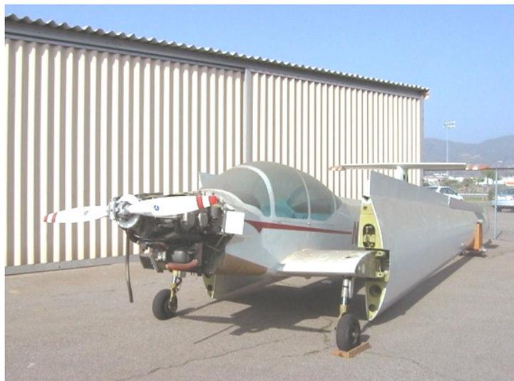
**ABOVE:** This is the Cloudster in its folded, hangered configuration. It has been in storage for a while after the start of an annual that hasn't been finished. It has an engine cowling and wheel pants, which make it look much sleeker when installed.
