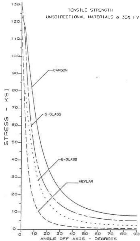
The next series of charts showed the tensile modulus of the four types of cloth at different volumes and formats. Modulus relates to the stiffness or deflection of the wing. It shows the degree of strength lost as the fibers get off-axis from the direction of tension. The numbers shown are those which should be attainable through normal layup and hand squeegeeing to the desired level of resin penetration.
