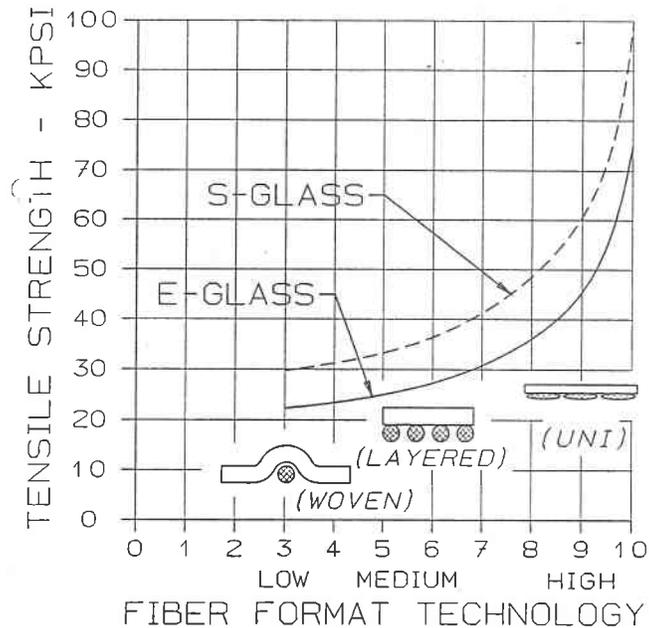
The chart showed that woven cloth at 30% fiber volume and 90° fiber orientation gives you about 22,000 psi tensile strength, but by using a layered cloth you increase this strength to about 27,000 psi. The uni fiber concept raises this to the 47,000 psi level simply by changing the format of the same weight of cloth.
