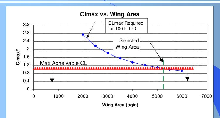
>Wing Area = 5300 sqin based on  $C_{Lmax} </= 1.0$
