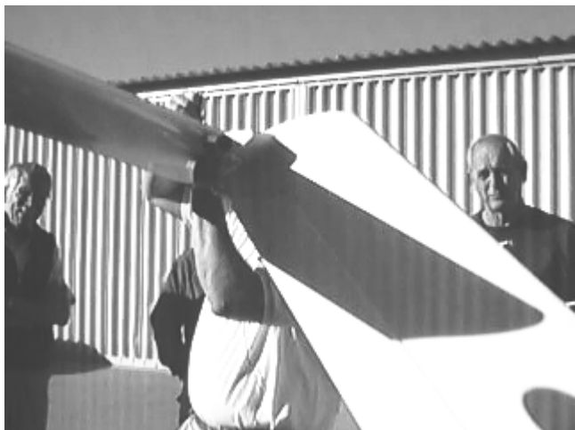
ABOVE: You can see Jeff's hand on top of the surface getting ready to pull up on the pin to slip it onto the horn. Note the leading edge is not yet all the way forward, which is also an indication the surface is not all the way on the control horn.
