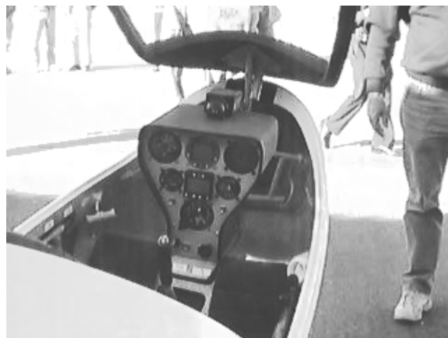
ABOVE: Shot of the instrument panel with programmable airdata computer resting on the top. You can also see that the cockpit is relatively roomy. The large cylinder on the right side of the canopy support is the jettison spring.
