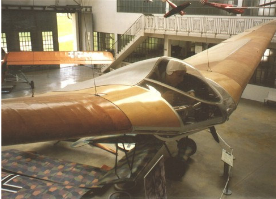
Flugwerft Oberschleissheim Horten IV after full restoration: old wings and new construction centerpiece. Picture by R. Storck.
