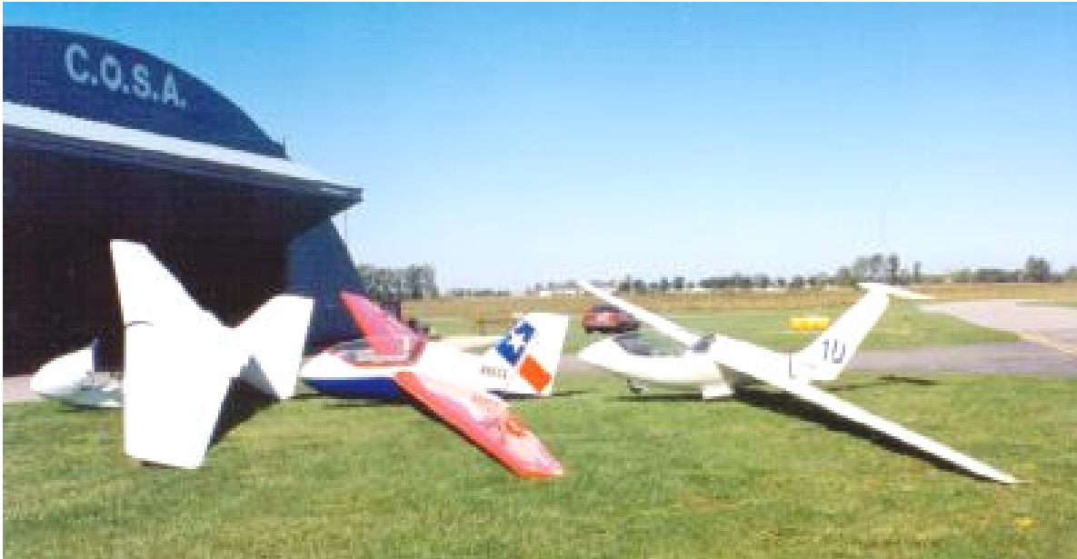
The Marske Monarch, Pioneer II and Genesis sailplanes on the ramp. Source: http://www.continuo.com/marske/index.htm
