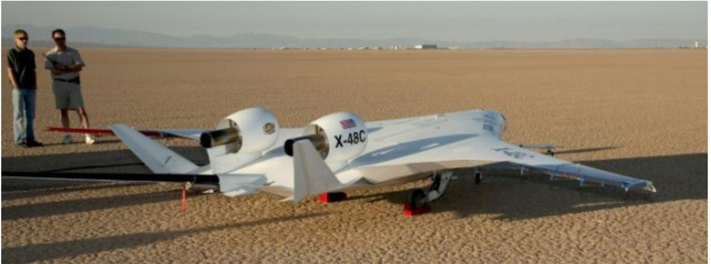
The X-48 is a Blended Wing Body aircraft, which is something of a halfway house between a flying wing and a conventional airplane. Note installation of larger engines than previous models.
