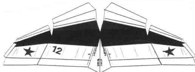
**ABOVE:** One of Pat's own designs. The upper lined areas are folded under the wing to form a rigid leading edge. The outer tips are then given some anhedral.
