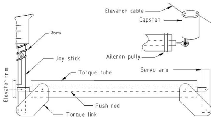
Either build it as if it were going to be in a tandem seating aircraft and leave the aft stick just a stub that you can use to run whatever mixer you're going to install.
