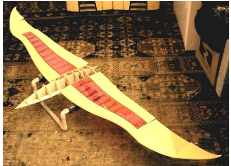
1mm x 28mm ply strip is cut to shape to follow the trailing edge curve and attached to the lower surface to give a sharp, strong trailing edge
