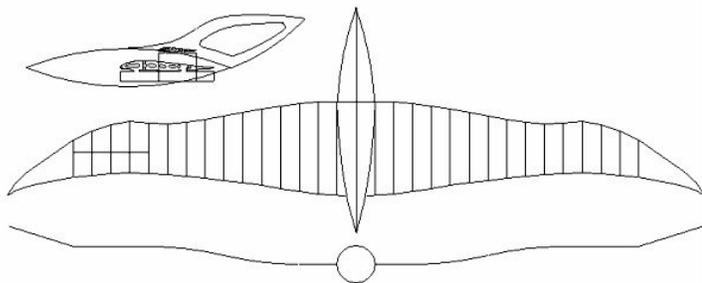
The ribs in the control surface area are aligned vertically so that the hinge line is straight and horizontal, this allows for top hinging.
