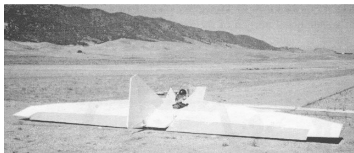
Waiting for tow at Tehachapi. Note the helmet. Les plans to make much smaller elevons on the second Primer.
