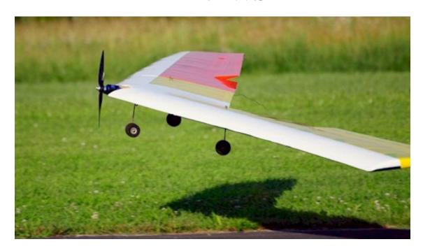
13 Foot Wingspan Flying Wing - Built from my own plans. Eppler 334 airfoil. 15 pounds with 6S 5000 mah lipo batteries. 50-65 brushless outrunner, 50 amp ESC, seven channels [elevons(2), throttle(ESC), pneumatic retracts(1), nose steering(1), drag rudders(2)] FLOWN Source: http://www.chrisgood.com/rcplanes/
