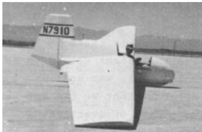
The landing flaps, despite their large size, were not effective when in ground effect. The glider could not be put down on the desired landing spot. Dropping the nose only increased the speed without any loss in altitude.
