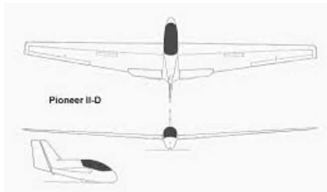
The initial Pioneer 2 version used a reflexed NACA 23012 profile at the wing root and a 23010 at the tip. While this aircraft performed well at high speed it did not seem to climb well in thermals. Later versions went back to the Pioneer 1's reflexed 33012 airfoil which was a definite improvement. The Pioneer 2 now climbed well and the high-speed performance did not seem to suffer.
