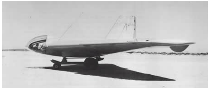
Fig. 10 A glider version of the XP-79 with detachable dollies for take-off.
