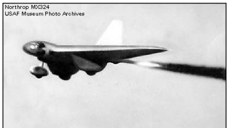
Fig. 11 Experimental version of the XP-79 with fixed landing gear shown during one of the early rocket-powered flights.
