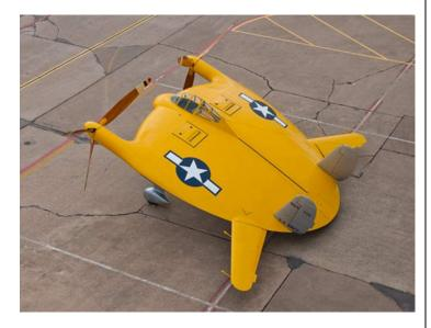
t still makes no sense to build in the extra complexity of the huge props (diameter and speed specifically designed to interact with the wing-tip vortices) when they first designed the plan form to maximize those vortices.
