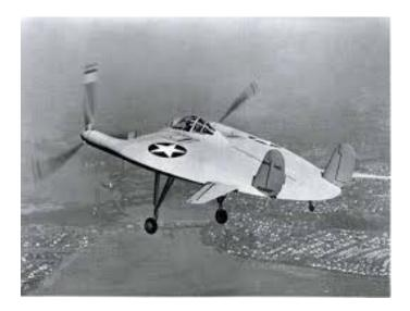
After seeing the Arup fly, Zimmerman settled on very nearly the same aspect ratio, as the most effective to maximize the wing-tip wash-around of the low aspect ratio plan form. After designing to maximize it, the Navy let them build on Zimmerman's flapping-prop idea for some reason, as if to improve efficiency and make it land slower.
