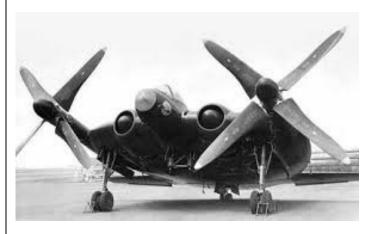
That would depend on the exact flight condition being tested. To get enough swirl in the propeller slipstream to cancel out the wing tip vortices significantly, it would have to be a flight condition with very high disk loading (so high power and low airspeed). The results you quote suggest they were using low disk loadings, so the swirl in the propeller slipstream was not having much effect on the intensity of the wing tip vortices.
