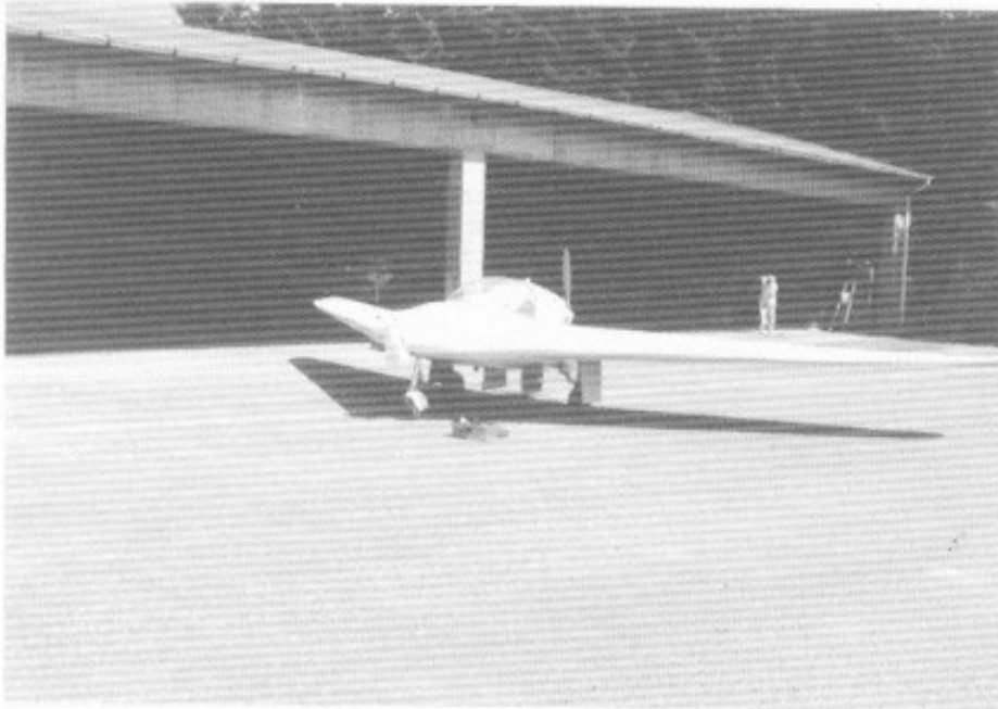
ABOVE: PUL-10 sitting in front of the hanger awaiting a test flight. Note the nose gear door and fender over the wheel to keep from throwing dirt and rocks onto the bottom of the wing. Picture by Barney Vincelette.
