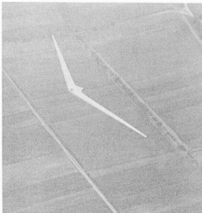
ABOVE: Let's have a little change of pace. Here is a view of the Horten IV in flight from above. Notice the high aspect ratio. Source: D. Bullard's website.
