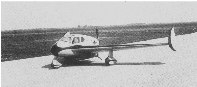
ABOVE: "Winged Flyer" - two-place, side-by-side tailless airplane. The tricycle gear was meant to keep the aircraft low to the ground so it could run as if an automobile. Pilot: P. Nadot. Circa 1945.
