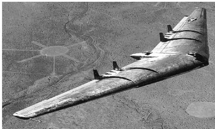
ABOVE: Northrop YB-49, eight engined, turbojet powered flying wing. Much sleeker and efficient than the XB-36 it was competing against.
