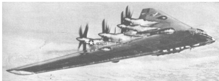
ABOVE: Northrop XB-35 which looks like the bigger brother to the N-9M, but with four engines and counter-rotating propellers.
