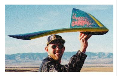
I've attached a PDF of Mike Allen's former web page. He explains how to build the right curve for a Klingberg Wing (above) with a Horten twist. It's not a straight line, and it's not a constant twist. Mike built the "fixture" as described out of foam core poster board. Then as he built the wing, he pinned the main spar to the fixture, and the trailing edge was pinned to the building board
