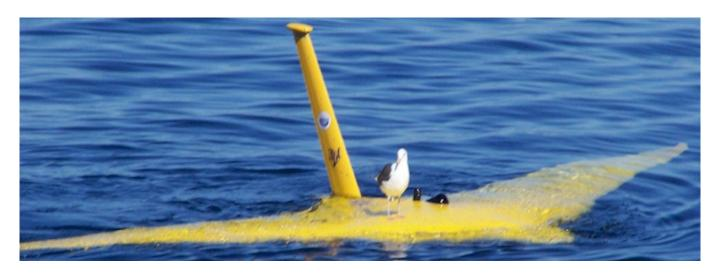
The 2007 version of the XRay2 Underwater Flying Wing glider being tested by the Scripps Institution of Oceanography. This could have both military and civilian applications as surveillance and survey vehicle. This view gives it a distorted look, but that is the water refraction effect. This will be the subject of our July 19, 2008 program.
