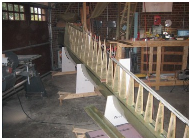
Adding built-up ribs and aft spars
