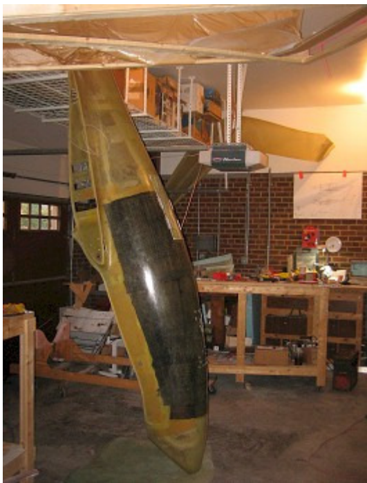
Tipped on end to mold nose tank for trim system
