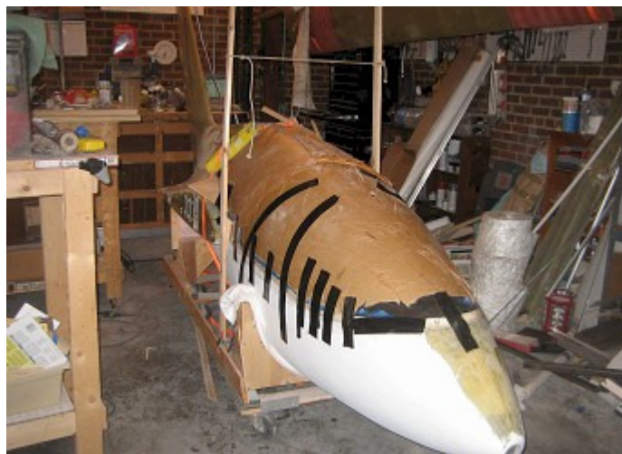
Transparency cut, fit, and epoxied to frame
