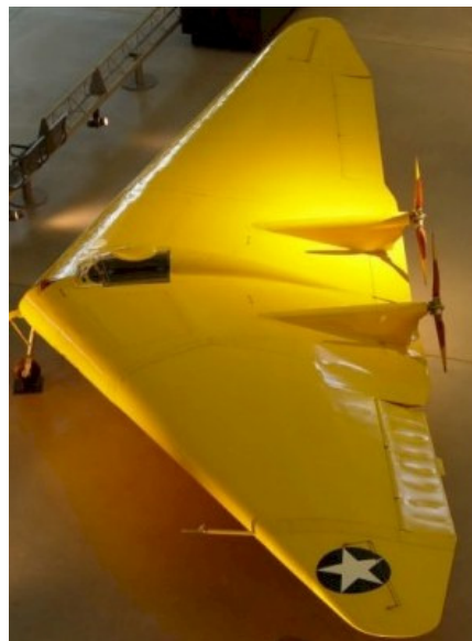
TWIN PUSHER —(Above) An early Northrop all-wing design was this little N1M single-seater of 1940, which had a span of 38.5 ft. and supplied valuable data for the XB-35 program. Power plants were two 65 h.p. Lycomings, later replaced by two 120 h.p. Franklin engines.
