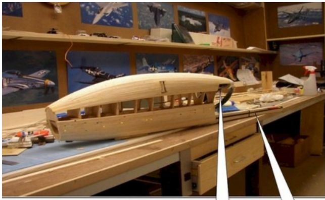
Fuselage being "Planked" When was the last time you planked a fuselage?
