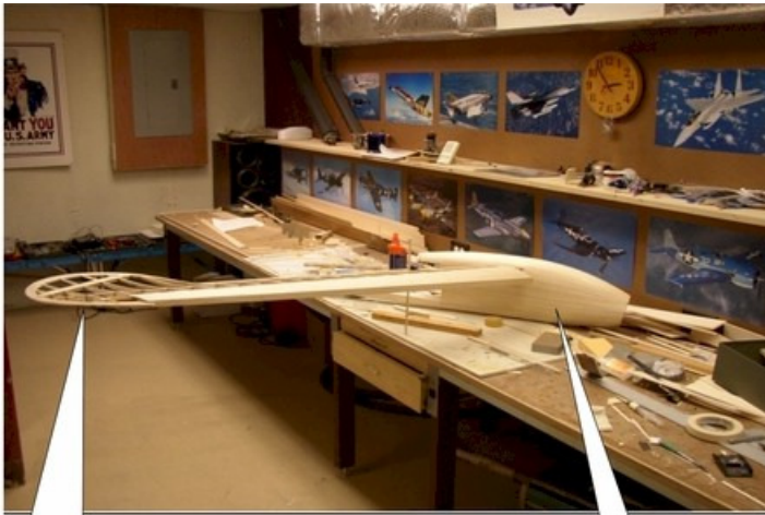
Right Wing Plugged into Fuselage
