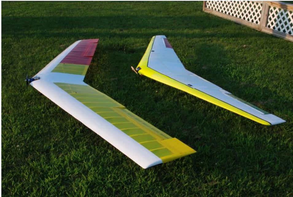
Electric Flying Wing (left wing) - 13 foot wingspan, Eppler 334 airfoil. Side by side with 11 foot Klingberg flying wing. Source: [http://www.chrisgood.com/rcplanes/wing\\_13\\_foot/index.htm](http://www.chrisgood.com/rcplanes/wing_13_foot/index.htm) for more construction photos. Outboard trailing edge appears to be split drag rudders.
