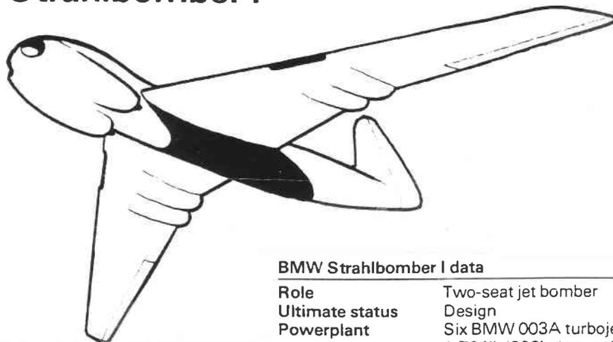
A pair of interesting bomber projects was produced by BMW under the designation *Strahlbomber* (Jet Bomber). Both were tailless and powered by the company's own engines. The *Strahlbomber* I was to be powered by six BMW 003A engines and had an apparently conventional fuselage and fin but no tailplane. The engines were located in pairs, one pair buried in each wing at about one-third span and the third on the nose, with one engine hung on either side of the lower fuselage.
