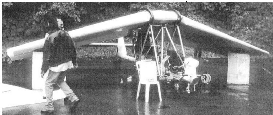
**ABOVE:** (I know, this doesn't have anything to do with this article, but it is the only place I could put it.) This is the Pneuwing from Peter's article during the deflation cycle. It is obviously a more conventional design, but shows how the pilot cage can be attached to the wing.
