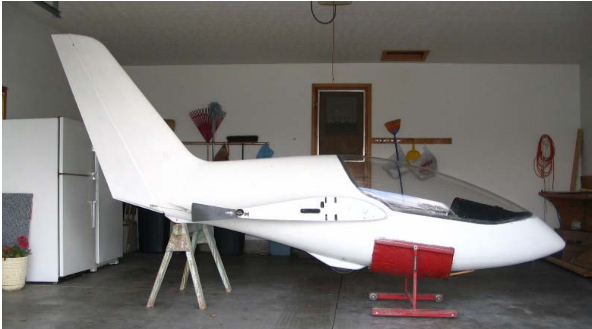
Pioneer III fuselage under construction by Jim Marske. First test flights may occur in May or June depending on how the weather cooperates for doing the finishing work. Beautiful lines. Source: http://www.marskeaircraft.com/flyingwings.html
