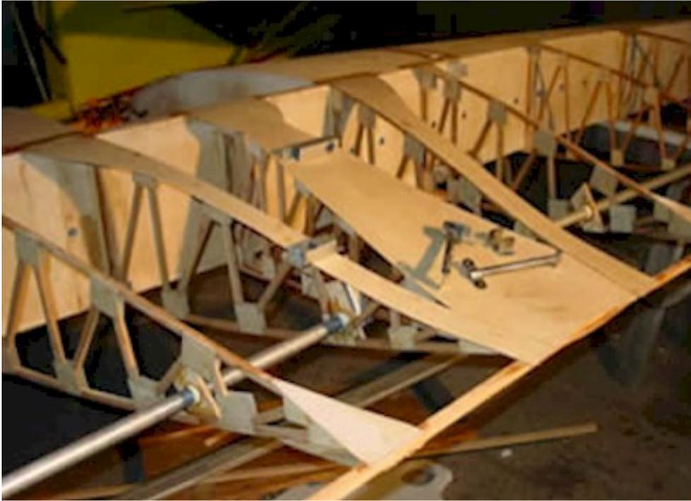
Wing center section. Note idler fitting resting on plywood and look at torque tube installation. I did not slit the PVC torque tube guides as per plans because they were plenty tight anyway.
