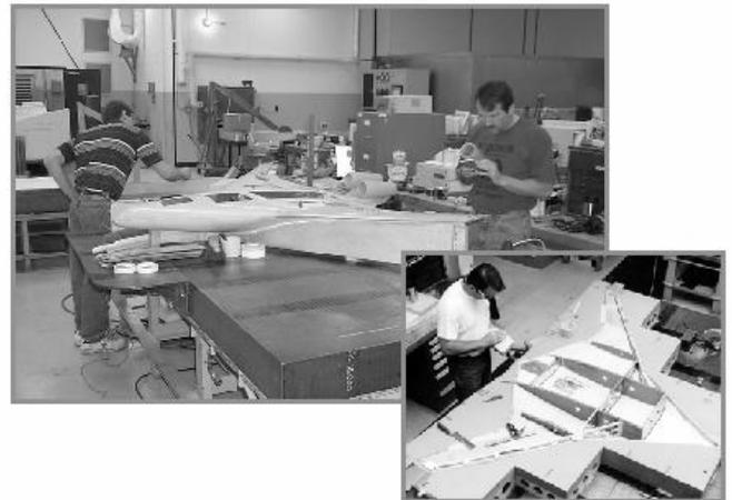
**3% LSV Wind-Tunnel Model Nears Completion**
