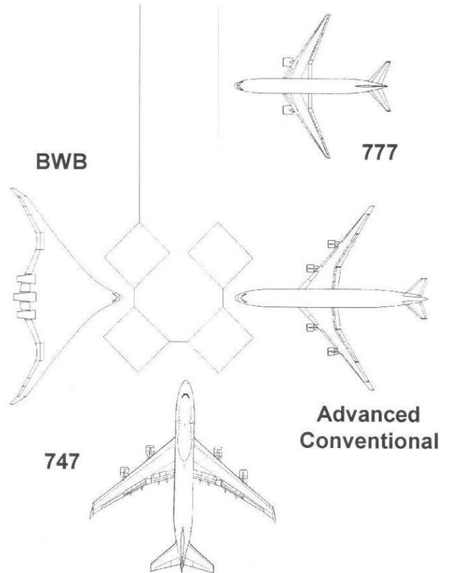
Al moved on to the infrastructure problems noted earlier (above). The ICAO wants to stay with the 80m (262 ft.) wingspan separation between terminal gates, so this becomes an intractable problem. The 800 passenger version was also a double-decker which presented another set of problems with the existing gate structures. The two decks also raised concerns over passenger safety in a crash situation where the upper deck could collapse onto the lower one. The last issue was how to
