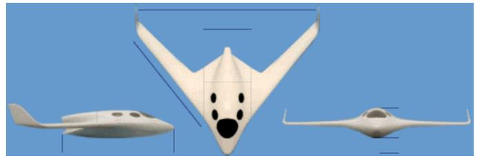
*The accompanying card contained some of the following information. Five-place, pressurized cabin [90"Lx80"Wx40"H], transatlantic range, stall resistant and impact safe airframe with chute. True 200 hour fuselage. Proprietary pressure molding. Many engine options and modular design. Complies with 51% rule. Phone: 321-253-1975 Fax: 321-253-3868 Address: 1425 General Aviation Dr., Melbourne, FL 32935. [www.wingco.com](http://www.wingco.com))*
