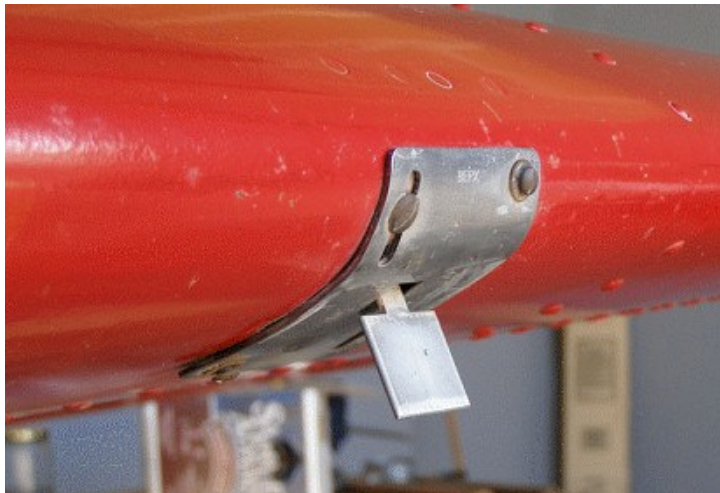
Yak 52 Stall Warning Tab (upper & lower)
