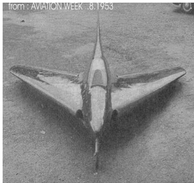
from : AVIATION WEEK .8.1953 FRONT VIEW of Payen P.A.49 shows experimental plane's delta wing and jet-engine air inlets on either side of fuselage.
