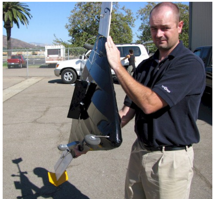
This is Dan holding the 2008 model that shows the belly flap deployed in the 90 degree position.
