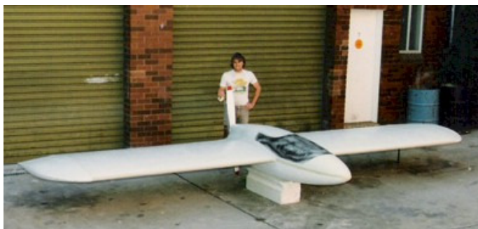
Facet Opal before installation of the vertical fins and landing gear.
