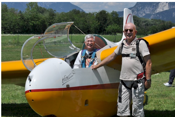
Above: Doug and Christian before their flight. Notice the black square on the fuselage about knee high on Christian. This is a footstep getting into the glider since the cockpit sill is so high.
