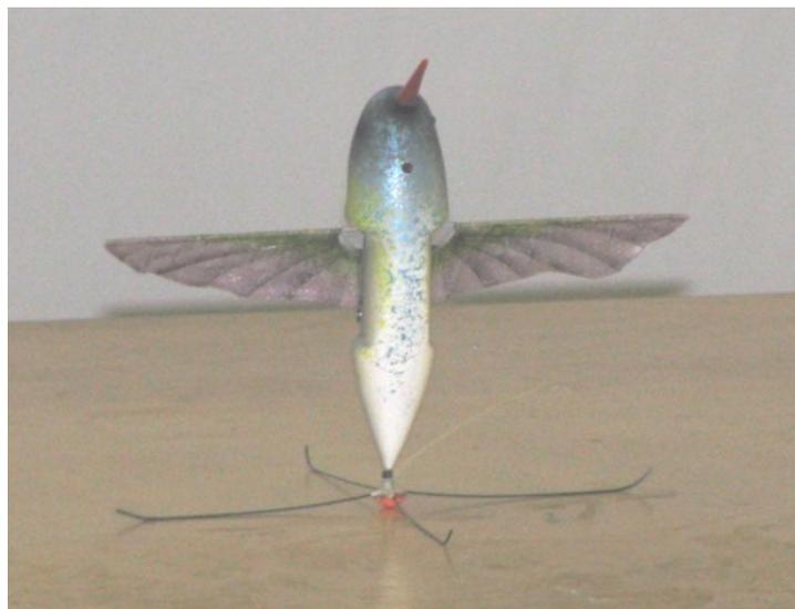
**Above:** Hummingbird on its launch stand (landing gear/legs). It is about 4" tall. It flew without the stand due to the high altitude at Tehachapi so you can see it is truly a tailless aircraft since the stand is not necessary for stability.
