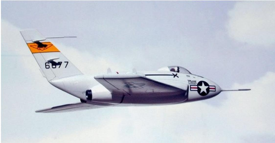
The Northrop X-4, Bantam, was a single-place, swept-wing, semi-tailless airplane designed and built to investigate that configuration at transonic speeds (defined as speeds just below and just above the speed of sound, but in this case, the testing was done primarily at just below the speed of sound).
