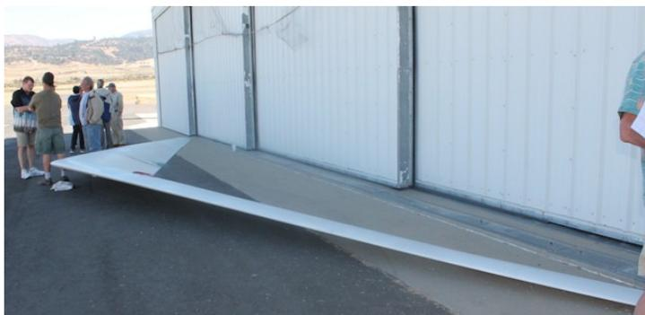
Complete wing that shows the degree of twist built into the wing panels.
